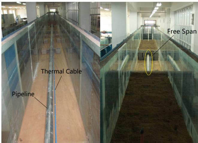
Fig. 2. Experiment setup.
